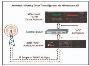
Wheatstone's ACI is a secure, proprietary TCP/IP-based network protocol designed for communication, monitoring, and control. For nearly fifteen years, ACI has found utility for interfacing not only Wheatstone products, but also other broadcast equipment: audio processors, consoles and surfaces, automation systems, and audio routers. The list of ACI-equipped Wheatstone products is long; if it's a Wheatstone product and it connects to a network, chances are it also has ACI built in.
